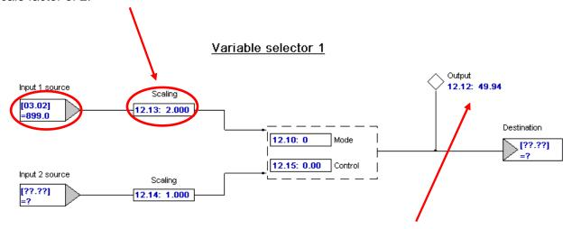
Shown above is a screenshot of an 1800rpm motor running at ½ rated speed or 900rpm. We can see 49.94% appear in the output of the Variable selector. The only problem is that this display could be a bit annoying as it will be flickering at a very high rate as #3.02 is updated. This could make the %Speed display readout un- usable. However, we could run this thru a Low Pass Filter to take the jitter out the signal and make it much more readable.
